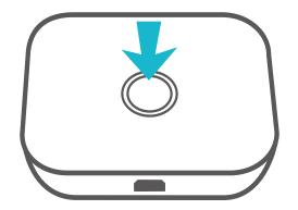
Keep pressing the power on button until the LED indicators lights up, which will indicate the Mobile WiFi is ON.
